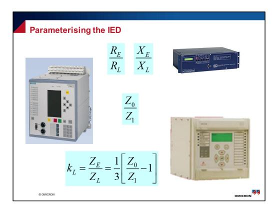
Re and Xe are the Resistive and Reactive reaches of the ground RL and XL are the Resistive and Reactive reaches of the phase
