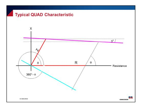
This is used mainly for earth faults where there is a high resistive component giving the IED a larger resistive reach. Related to arcing or tower footing or if the return path is highly resistive.
