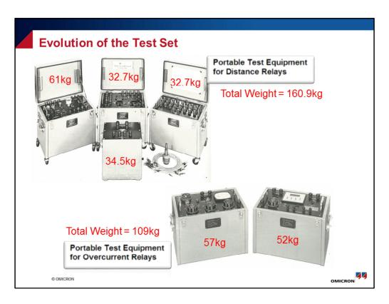
1<sup>st</sup> pic – GEC ZFB – full of copper and Iron, was state of the art until the late 70's, it's a distance protection test set (impedance test set)
