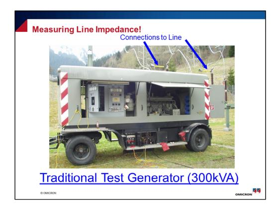
In the past, when unsure about Line Impedances there was a requirement of a large generator to make the measurement at line frequencies. This size was to overcome effects of surrounding noise, effects of cables etc
