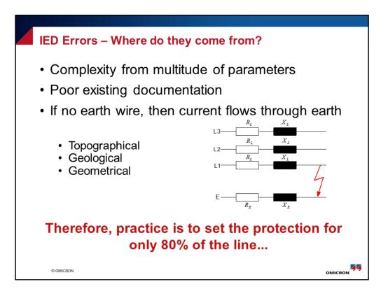
Complex – at system design, errors in calculations Docs – old sub stations may lose documentation CT/VT accuracies Geometrical – geometery of the power system
