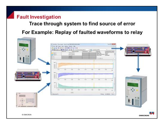
Very often BAD things happens and faults are developed. Here we see 3 different types of kit that can be used for fault investigation.
