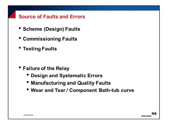
SCHEME FAULT – something in the design that causes the IED to operate when it should not, ie blocking scheme
