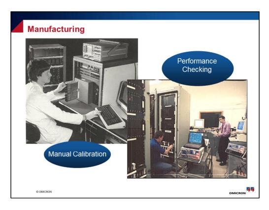
Old mechanical relays were calibrated using trim pots for adjustment, this is a pic from the early 1980's showing how it was done.
