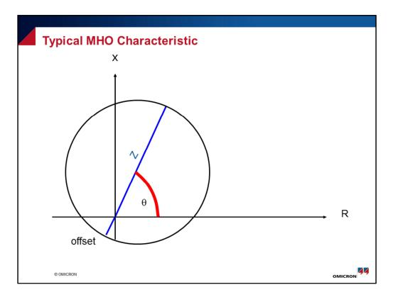
this is defined by the impedance of the line and the line angle it has an off set indicating that the IED is directional looking forward along the line and also looking in the reverse direction by a certain distance.
