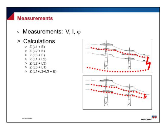
Calculates the different fault loops
