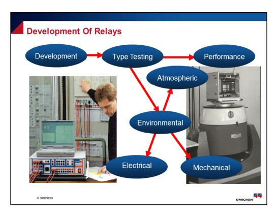
TYPE TEST – after development of products it is usually standard to have it approved by a regulating Testing Authority to ensure that IED is safe and operates as desired and suitable for the network, ie Fast Transient testing
