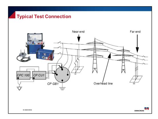
•We are not connected directly to the lines and the GB1 has safety surge arrestors if any line coupling occurs.
