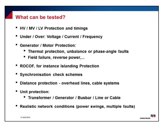
ROCOF – rate of change of freq – measures how quickly the freq reduces – monitoring a generator freq at overload and see how quickly the freq reduces rather than wait until the freq reaches a defined low level resulting in the removal of the generator from the grid before any damage can occur.
