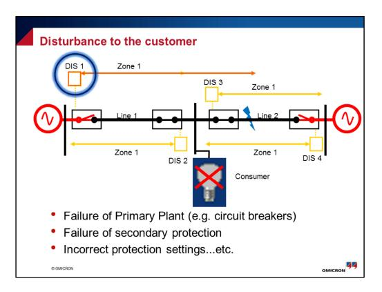
When a fault occurs on Line 2 the fault is seen in Zone 1 by the IED DIS 3 and DIS 4
